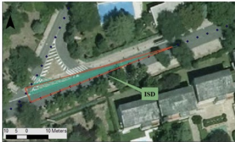
Fig. 7. Departure sight triangle for the minor road
