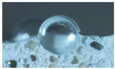
Fig. 2. Cross-section of a road marking material with a properly embedded glass bead
