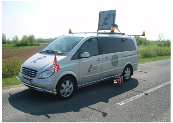
**Fig. 3.** *Vehicle with side-mounted retroreflectometer*
