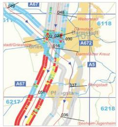
**Fig. 6.** *Example of a thematic map with condition data of road surface*
