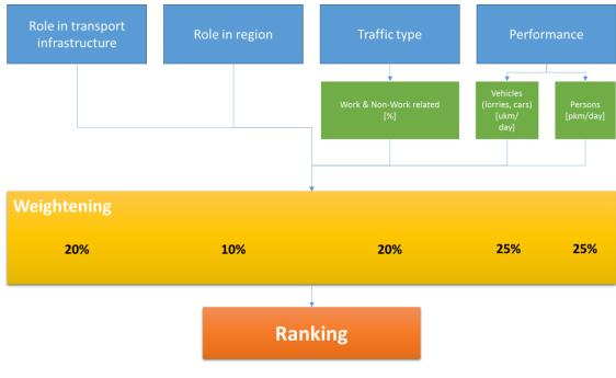
Fig. 3. Concept of decision support tool Source: own compilation
