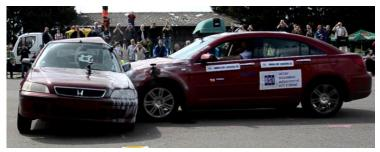
Fig. 3. Side crash test between Chrysler Sebring (moving vehicle) and Honda Civic (author)
