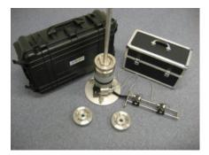
Fig. 1. Light Weight Deflectometer
