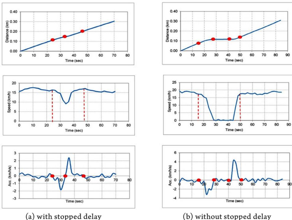
**Fig. 4.** Examples of Speed Profile, Time-Space Diagram and Acceleration Profile with and without Stopped Delay
