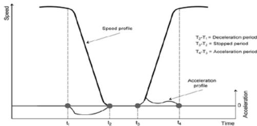
(a) Speed profile with stopped delay
