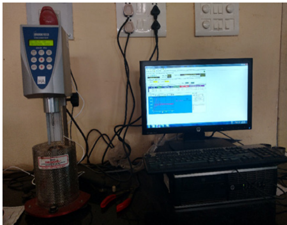
Fig. 4. Brookfield DV-II Pro Rotational Viscometer Source: (Own Source)
