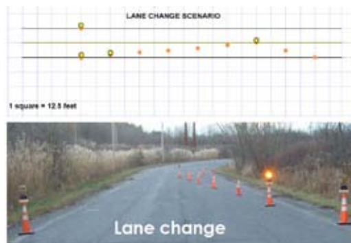
Fig. 4. Plan View Layout (Top) and Photograph (Bottom) of the Lane-Change Simulated Work Zone with the Right Lane Closed
