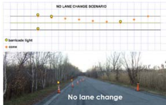
Fig. 3. Plan View Layout (Top) and Photograph (Bottom) of the No-Lane-Change Simulated Work Zone with the Left Lane Closed
