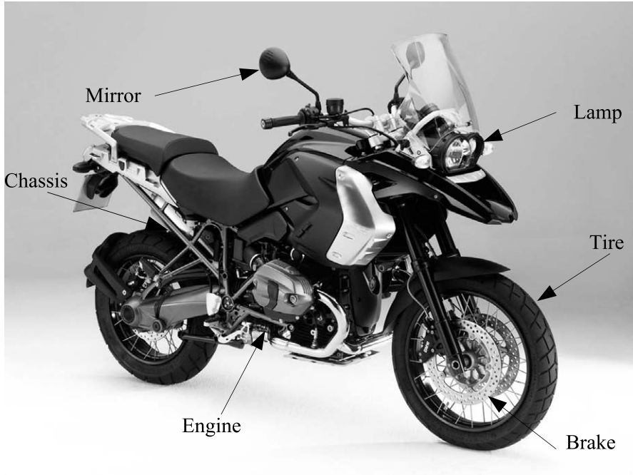
Fig. 1. The Main Components of a Motorcycle Source: Author
