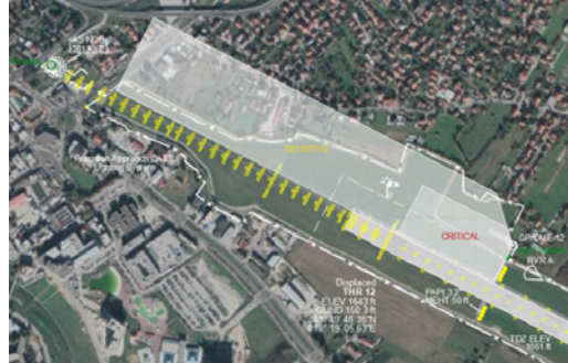
Fig. 3. CAT I Critical and Sensitive Area for Sarajevo Airport Runway 11 Source: Own Edition
