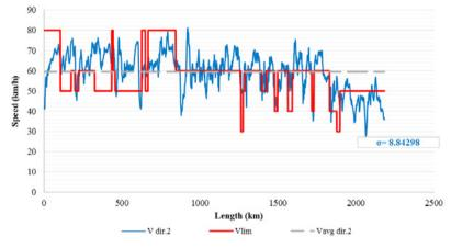
**Fig. 8.** Speed Profile on the Section Mali Zvornik - Gračanica in Direction 2 (11/11/2018 at 12.02p.m)
