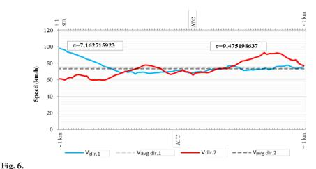
Speed Profile for ATC Zone on the Section Čačak (Guča) - Pakovraće (Markovica) (April 4, 2019 at 9. 16 a.m. & 11.33 a.m)
