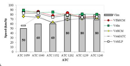
**Fig. 3.** *Relationship between Free Flow Speeds (Linear and HCM), Operating Speeds (Linear, HCM, Modified Linear Procedure - MLP and Actual Operating Speeds from ATCs) and Limited Speeds*
