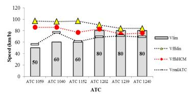
**Fig. 2.** Relationship between Free Flow, Limited and Operating Speeds Read From ATCs
